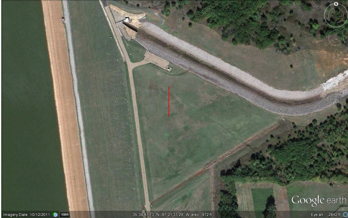
Figure 6.2 - Location of 57.5m Arcadia Dam MASW survey directly east of Arcadia Dam, depicted by the red line. The edge of Lake Arcadia is shown on the western edge of the picture, and the spillway is shown to the north and east of the survey line. Image courtesy of Google Earth.
