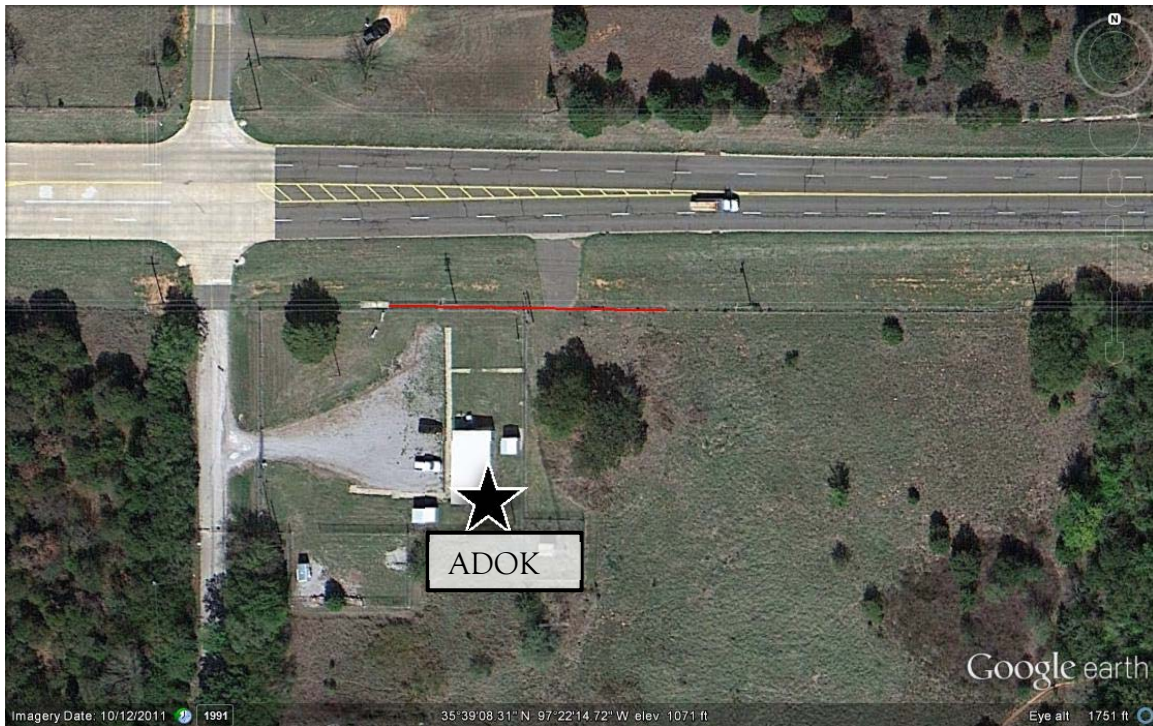
Figure 6.1 - Location of 57.5 m ADOK MASW survey by OGS seismic monitoring station, depicted by the red line. The shown intersection is of Old Route 66/Edmond Rd and S. Douglas Blvd in Edmond, OK. The building is the Army Corps of Engineers Arcadia Dam facility. Image courtesy of Google Earth.
